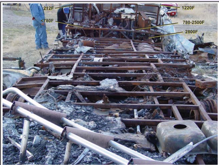
Fig. 14 Overall view of recreational vehicle with approximate maximum fire temperatures noted
