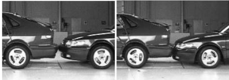
Figure 2. 1999 Saab 9-3 precrash (left) and mid-crash (right)
