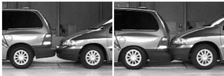
Figure 1. 1999 Ford Windstar precrash (left) and mid-crash (right)
